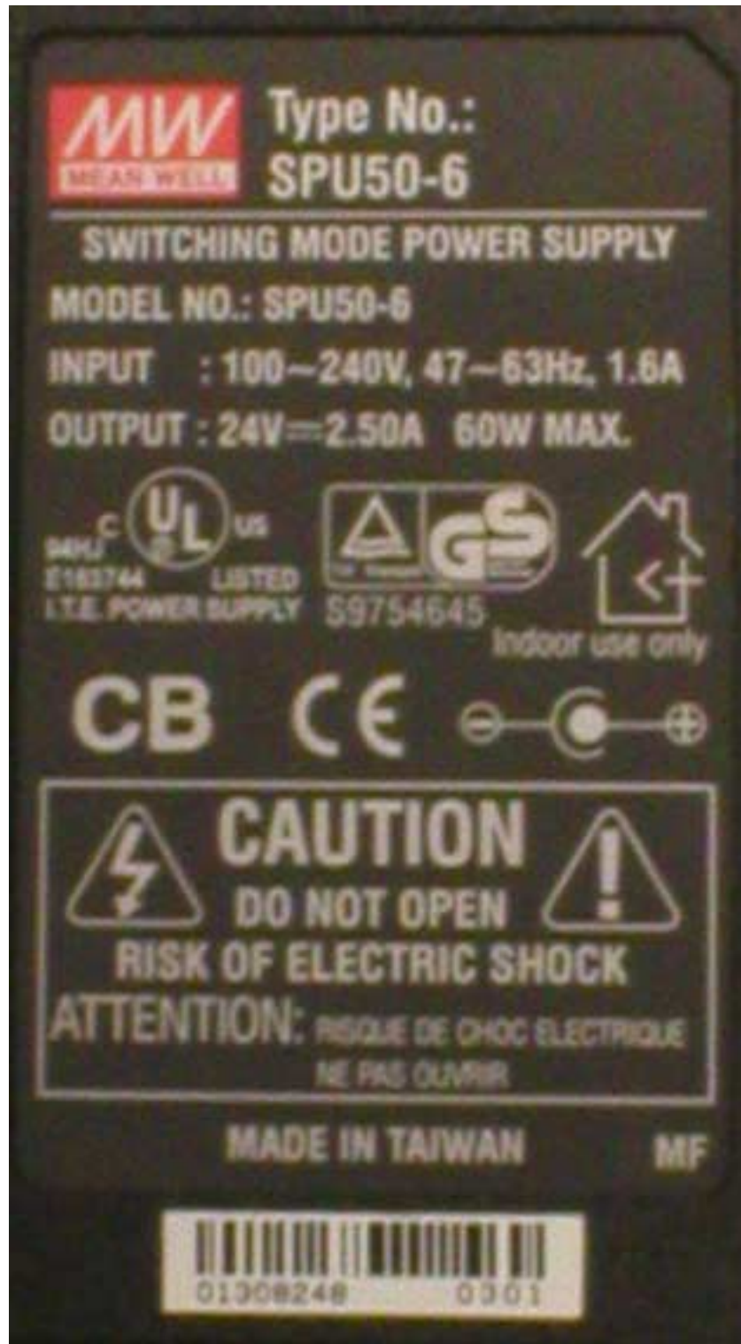
Figure 7: Power Supply Label
